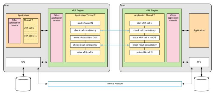
Figure 2 – Consistency Checking Between Two Replicas
